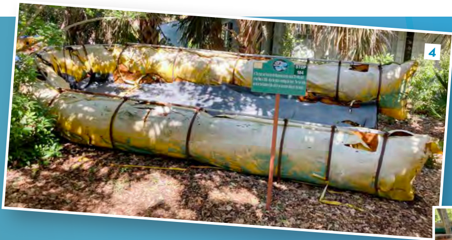
4 Vessel #4 features hand-sewn tarpaulins, spray foam, iron bands and hoops, gray plastic matting, and iron barrels that acted as integrated fuel tanks. The latter presumably powered the missing outboard engine.
