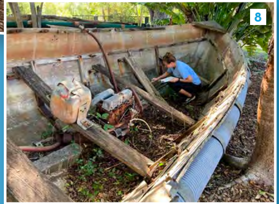
8 Vessel #8 is fashioned from aluminum panels and may have had six benches for seating. The inboard Nissan diesel engine was fueled from a plastic tank mounted on a thwart. The vessel also features a modified exhaust pipe that likely produced the distinctive “chug chug” sound that for which these vessels are known.
