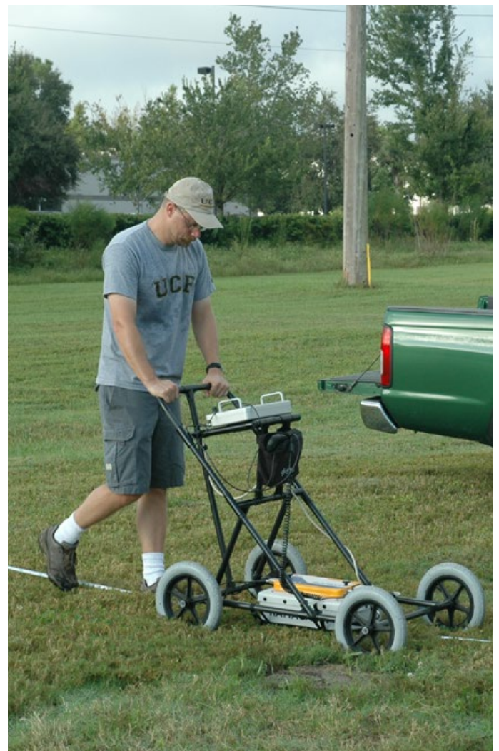
Dr. Schultz pushing the GPR unit over a grid line during a research project.
